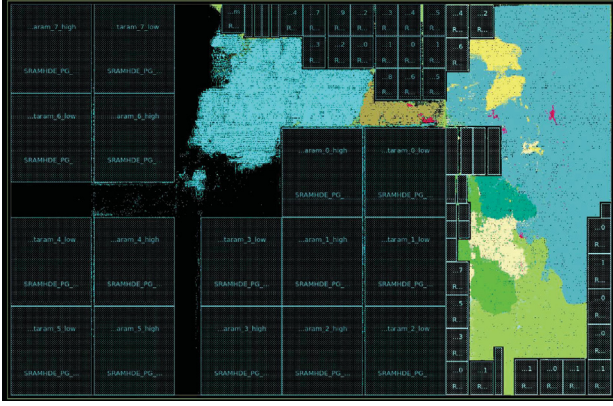
Figure 7: Microprocessor layout with DEEP component-level OPM integrated. The red region is OPM. Area overhead AO_L = 0.04\% when measured on this layout. The MAE = 9.5% and R = 0.954 .
