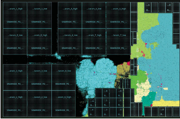
Figure 8: Microprocessor layout with state-of-the-art baseline B1 [38]-OPM. The red regions is OPM. Area overhead AO_L = 0.16\% . The MAE = 9.5% and R = 0.951 . Its overhead is 4 \times of the DEEP solution.
