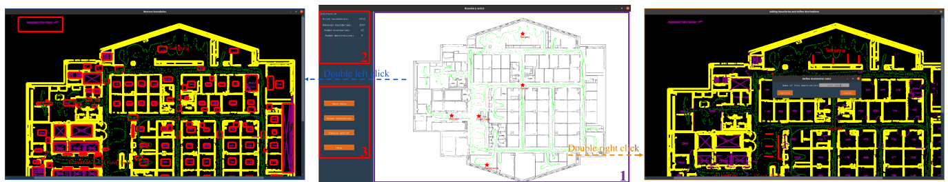
Figure 5. Boundary/destination GUI. The main window is displayed in the middle . It comprises three zones. The green dots in Zone 1 depict the locations of database images, while the red star indicates potential destinations. After double-clicking Zone 1 , map-makers can adjust boundaries and desired destinations in additional pop-up windows ( left and right ). After double left-clicking Zone 1 , the map-maker can delete boundaries in the pop-up window ( left ) by removing line segments (which represent boundaries) using an edit tool (red superimposed box). After double right-clicking Zone 1 , another pop-up window ( right ) will appear, in which the map-maker can draw red lines to represent additional boundaries and define potential destinations by clicking green dots and assigning destination names to them. Additionally, boundaries and destination information are provided in the Zone 2 ( middle ). Once all the boundaries and destinations are defined, the map can be saved in Zone 3 .
