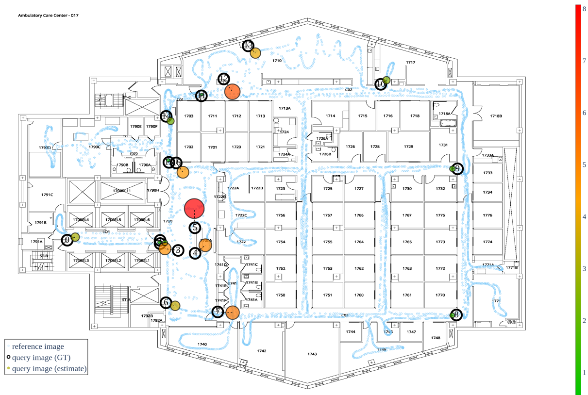
Figure 9. Location accuracy heatmap. The small open light-blue dots are the locations of n reference images on the floor plan. The open black circles are the ground truth locations of 17 testing images; the multi-colored circles next to the GT localizations colored from green to red are the estimated locations of these 17 testing images; the further from the ground truth location (ft), the larger the circle and the warmer the color (red).
