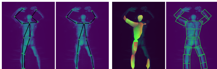
Fig. 1: Example of our refined 2D pose (2 nd ) and unsupervised body segmentation (4 th ) on MWS images compared to SOTA HRNet 2D pose (1 st ) [28] and DensePose body segmentation (3 rd ) [14].
