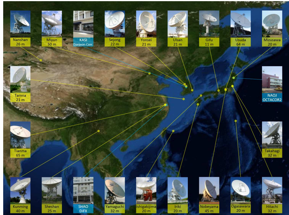
Figure 1. Concept map of EAVN including 16 active telescopes listed in Table 1, three potential telescopes (Miyun 50 m in China, Gifu 11 m, and Usuda 64 m in Japan), and three correlator sites in China, Japan, and Korea. Photographs of each radio telescope and correlator site are overlaid on ‘the Blue Marble’ image (credit of the ground image: NASA Earth Observatory ( https://earthobservatory.nasa.gov/ ), accessed on 1 December 2022).
