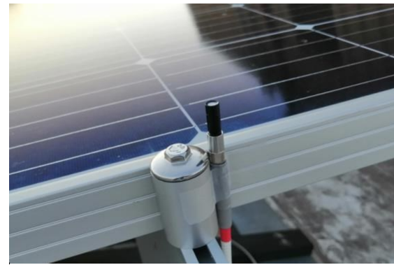
Fig. 4. Solar spectra data acquisition system setup.
