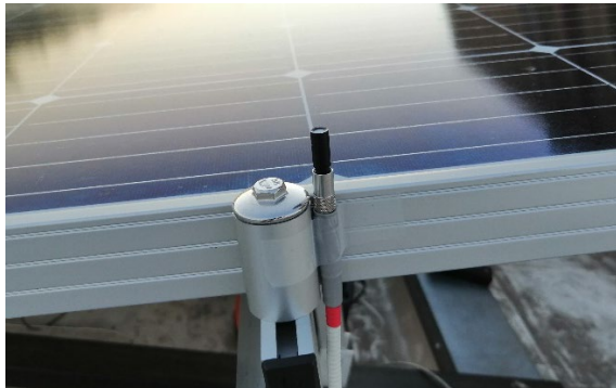
Fig. 10. Solar spectral irradiance measurement setup on the PV panels.
