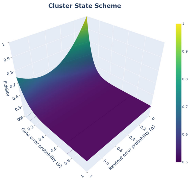
Fig. 15 Final state fidelity surface plot from a three-qubit teleportation scheme with varying depolarizing noise, p , and intermediary readout dependent error, q , following Eq. (17) and the coefficients of (19)
