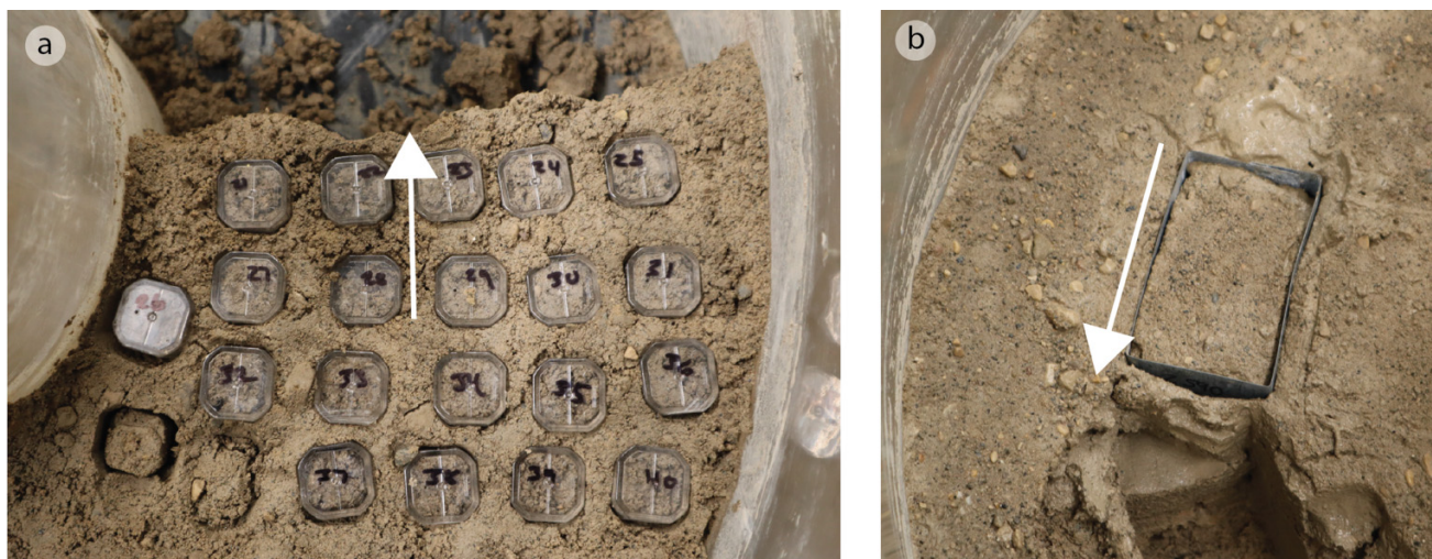
Fig. 5. Sample collection following the completion of the experiment. (a) AMS sample collection from 2–4 cm depth interval. The white arrow denotes the direction of ice flow. (b) Microstructure tin placed in the till prior to extraction for the 0–4 cm depth interval from which thin section 1 (TS1) was produced. Ice flow is in the direction of the white arrow.
