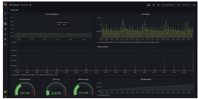
Fig. 5. A Grafana panel showing system statistics data. It is showing the real time status of the Raspberry Pi 2. From the picture, we could monitor the CPU core temperature, Memory usage, CPU short/long term load and disk usage, etc.
