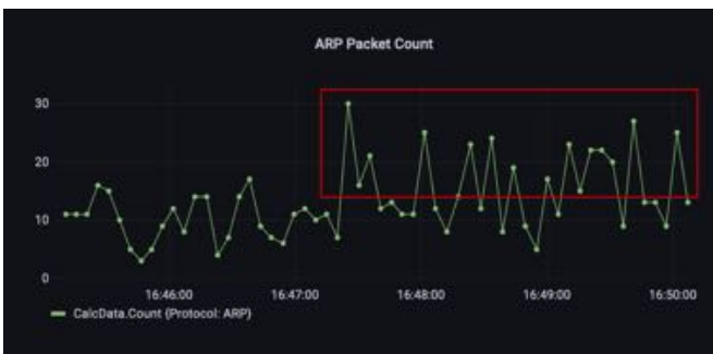
Fig. 4. A Grafana panel showing ARP Packet counts. Note the increase in ARP traffic during an attack highlighted in the red box.
