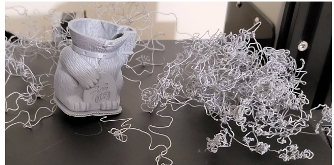
Figure 2: A classic print failure is the so-called ‘spaghetti’ print, shown here. If a print moves partway through printing, the nozzle will extrude filament mid-air, creating clumps of plastic which look like spaghetti. Image from r/FixMyPrint.
