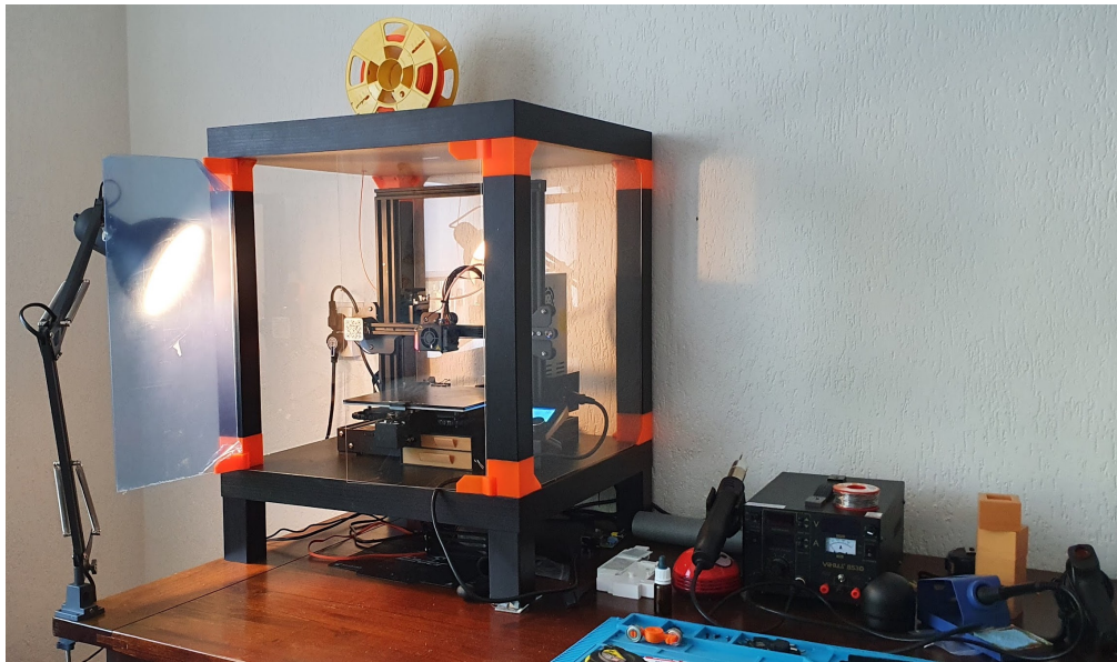
Figure 4: P1's home printer setup. In our video interviews, participants shared their home printing workspaces with us. One of P1's first projects was 3D printing parts to make an enclosure for their Ender3 Pro; this helps maintain a closed environment to minimize environmental impact on prints. Apparent in the image is the 3D printer housed in this custom enclosure. P1 is interested in hobbyist electronics and often 3D prints enclosures. An electronics workstation including a soldering iron and power supply is visible next to the printer. Underneath the enclosure we can see a Raspberry Pi which P1 has set up with their printer to run OctoPrint [26], a software which allows remote control of 3D prints.
