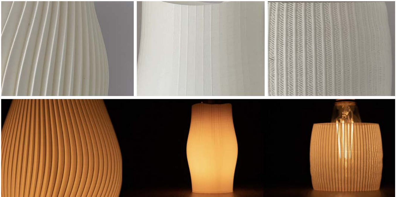
Figure 6: Lampshades printed with Vespidae. The two lampshades to the left were printed with non-planar printing program shown in Figure 5. In that program, we can parametrically vary the pleating, the non-planar layers, and the lamp’s radius at different heights. The rightmost lampshade was printed by extending this program with the Pulse Extrude-Action described in Section 5.2, Flexible 3D Prints Through Under-extrusion. This introduced additional transparency and flexibility in the shade. We experimented extensively in order to find good input values for extrusion amount and frequency of pulsing. The challenge was to extrude enough for sticking, yet not so much as to result in a solid print. Being able to quickly export and execute G-code on our printer allowed us to focus on the material exploration aspects rather than on moving files around.
