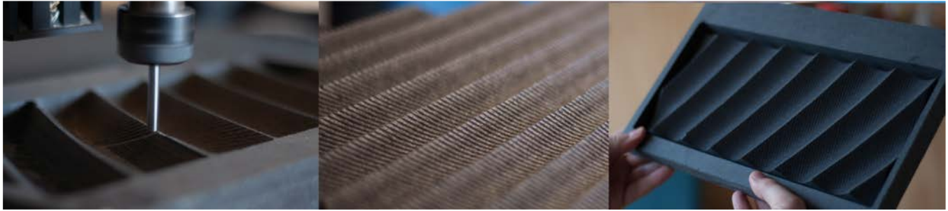
Figure 8: Results from our experiments milling Valchromat using a Vespidae program with Cut-Actions. The ridges, tool marks, and machine speeds and feeds are all parameters we experimented with.
