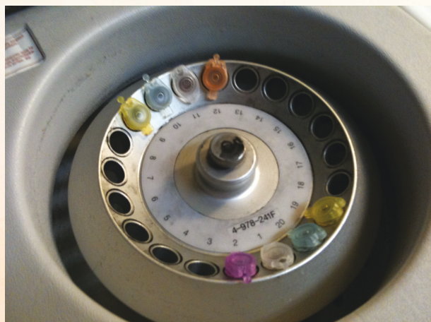
Figure 1. A 20-hole balanced centrifuge with 8 test tubes.
