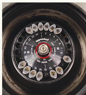
Figure 2. A 24-hole balanced centrifuge with 13 test tubes.
