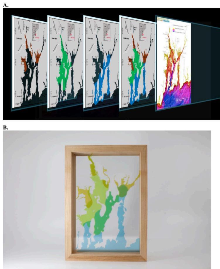
**Figure 4: The second physical framework of three theoretical zones in Narragansett Bay. (A)** The schematic images of the entire three zones in the Bay for UV printing and stacking of the second physical framework. **(B)** The framework created using four acrylic sheets to show overlaps of zones' boundaries. [Please click here to view a larger version of this figure.](#)
