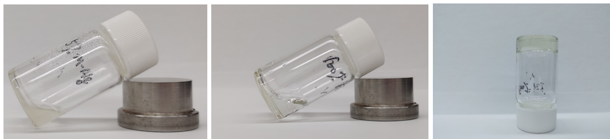
Figure 7. Hydrogel formation by mixing alginate-GlcN solution (left) and branched poly(ethylene imine) solution (middle) to form the hydrogel depicted on the (right).
