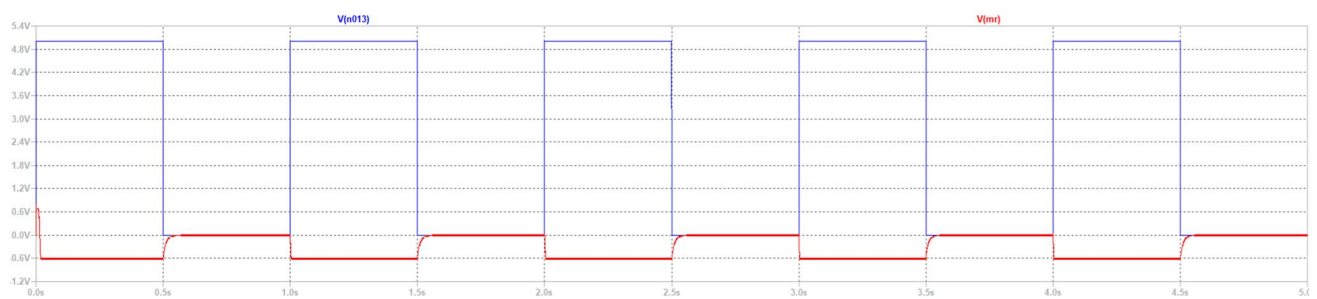
Fig. 17 Case 2: Original message ( V(n013) ) in blue color and decoded message V(mr) in red color
