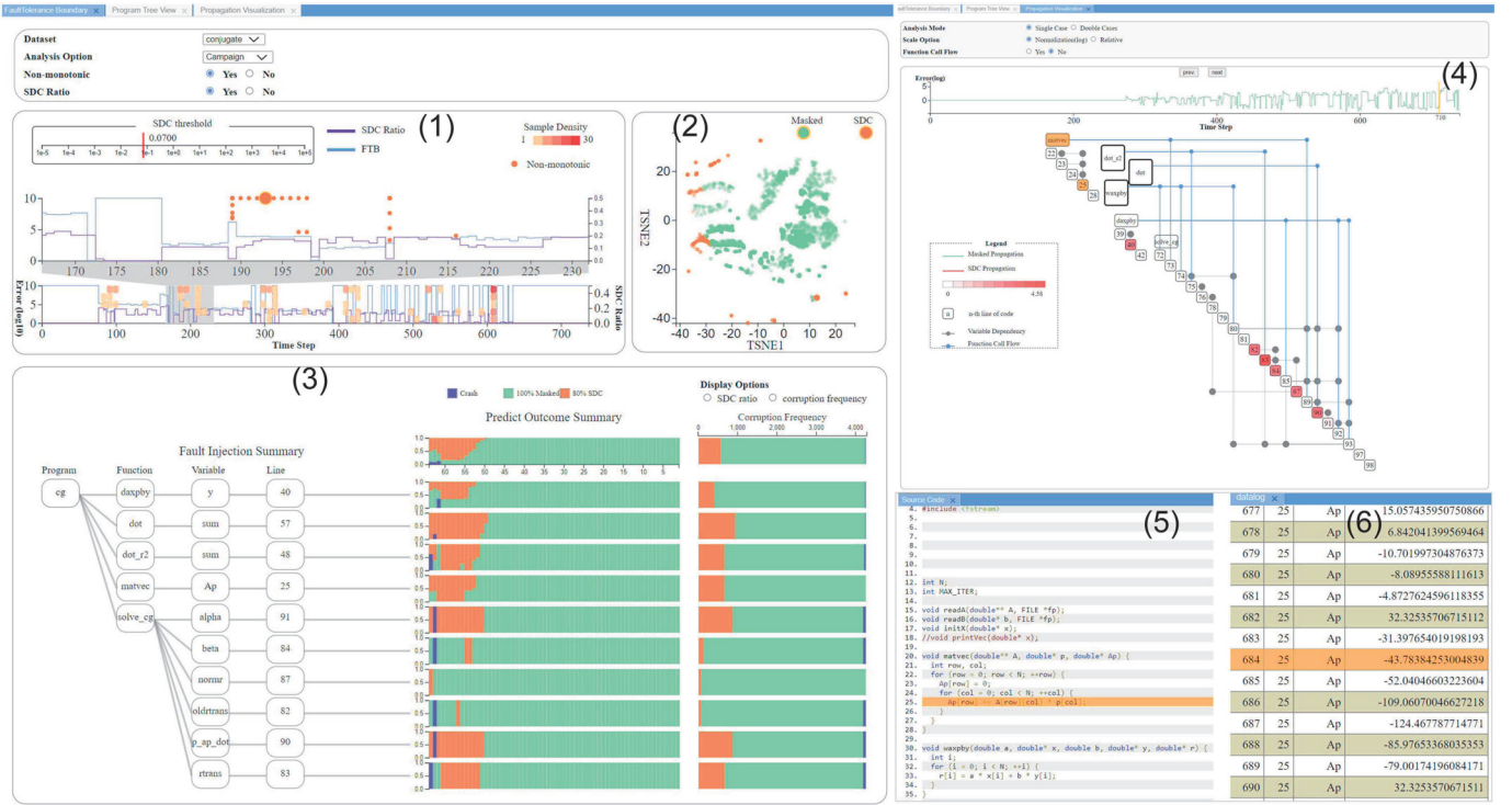
Fig. 1. View (1) on the left shows a fault tolerance boundary visualization of the conjugate gradient algorithm. An execution interval is selected in the boundary view, and the related bit-flip outcome over each bit in the interval is displayed in (3). The error propagation that starts from the selected interval is highlighted in view (2), and similar error propagations are clustered together. Views (4), (5), and (6) on the right coordinate with each other to demonstrate a nonmonotonic error propagation case in which a large error is injected in the middle of the program but mitigated.
