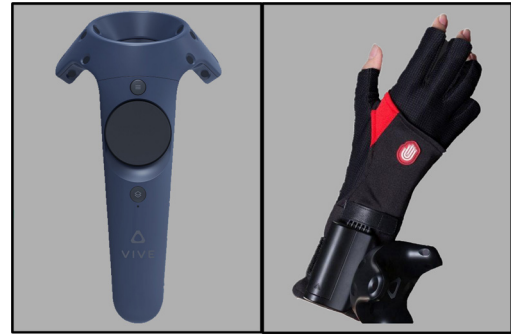
Fig. 2: The input devices used in the experiment. a) HTC Vive Pro controller, and b) Noitom's Hi5 VR glove
