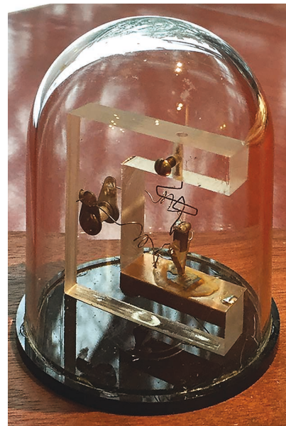
FIGURE 1. An early reproduction of the first point-contact transistor. This replica is on display at the Holonyak Micro and Nanotechnology Laboratory at the University of Illinois at Urbana-Champaign (on loan from Prof. Jont Allen).
