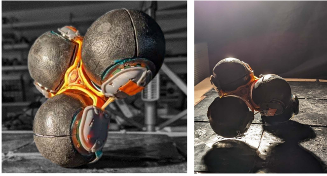
Fig. 1. FireAntV3 improves upon previous robots both through updated mechanical design as well as through expanded sensory capability. Each robot sphere is 65 mm in diameter.
