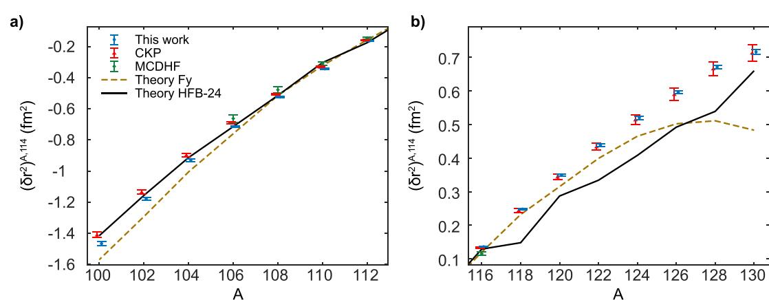
**Figure 4.** Squared RMS charge radii of even–even Cd isotopes relative to  $^{114}\text{Cd}$ . (a): proton rich, (b): neutron rich. The data points correspond to columns 2–4 of table 4. The nuclear theory lines are from the Fayans functional (Fy), extended by information on the radii of Ca [56], and Skyrme–Hartree–Fock–Bogoliubov mass formula (HFB-24) [39].
