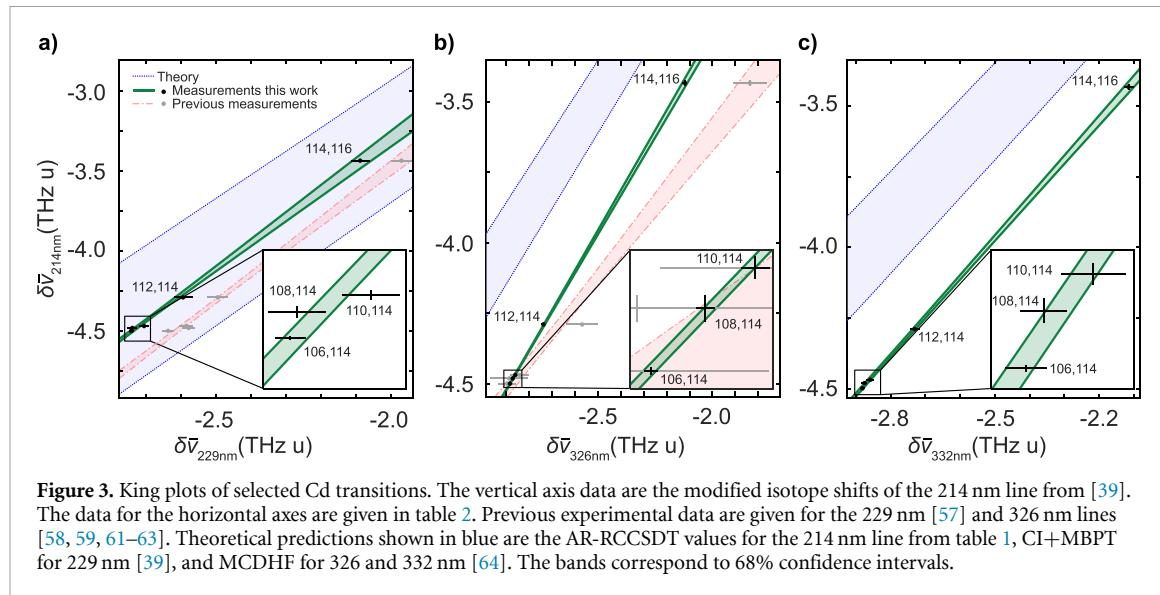
**Figure 3.** King plots of selected Cd transitions. The vertical axis data are the modified isotope shifts of the 214 nm line from [39]. The data for the horizontal axes are given in table 2. Previous experimental data are given for the 229 nm [57] and 326 nm lines [58, 59, 61–63]. Theoretical predictions shown in blue are the AR-RCCSDT values for the 214 nm line from table 1, CI+MBPT for 229 nm [39], and MCDHF for 326 and 332 nm [64]. The bands correspond to 68% confidence intervals.
