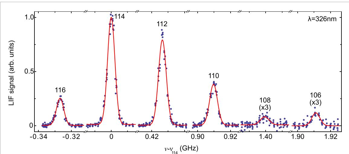
**Figure 2.** Isotope shifts of the Cd I bosons at 326 nm, measured with a cryogenic helium-cooled atomic beam and a frequency-doubled dye laser. The fermionic hyperfine transitions are beyond this spectral range.
