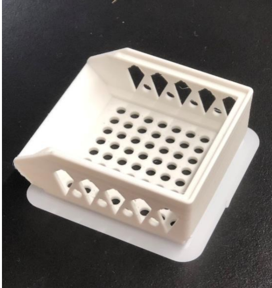
Figure 1. Photograph of the model that was printed with a four hour print time using the three test filaments in this study. The model in this figure was printed with the ABS filament and measures 53.6 x 61.9 x 25.0 mm. Masses of models varied depending on the printing time and the filament used.
