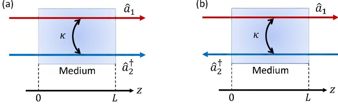
Figure 1. Schematics of two coupled phase-conjugated electromagnetic waves: (a) forward-wave configuration, and (b) backward-wave configuration.  $\kappa$  is the nonlinear coupling coefficient between the two modes.
