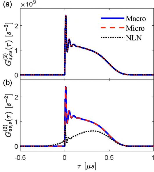
Figure 9. Two-photon Glauber correlation in time domain in the group delay regime: (a)  $G_{s,as}^{(2)}(\tau)$  and (b)  $G_{as,s}^{(2)}(\tau)$ . The simulation conditions are the same as that in Figs. 3, 4, and 5. NLN: no Langevin noise included.
