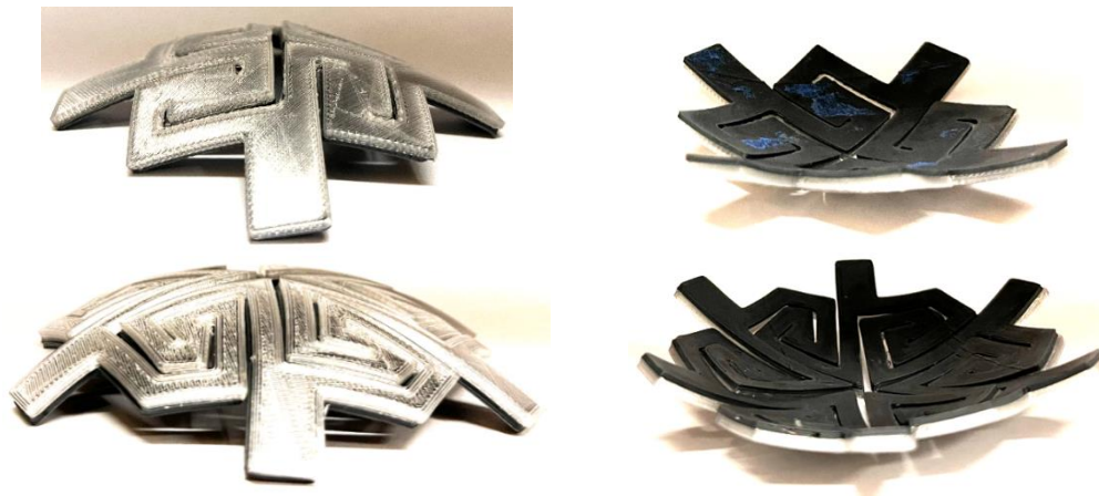
Figure 11. Deformed shape of bilayer square (top) and hexagonal (bottom) kerf cell subjected to thermal load
