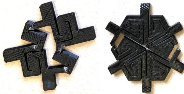
Figure 7. PLA square (left) and hexagonal (right) kerf unit cells after failure
