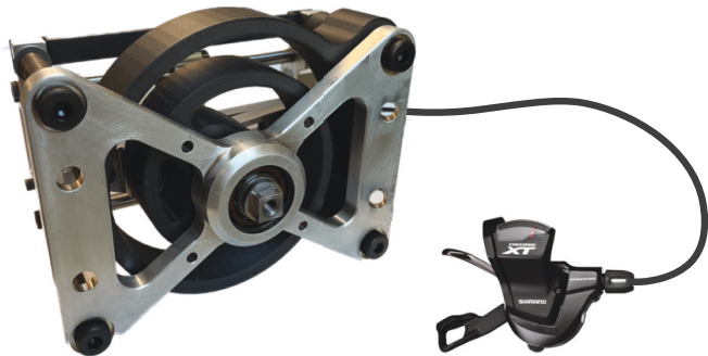
Fig. 1. Variable stiffness spring with human-selectable stiffness.
