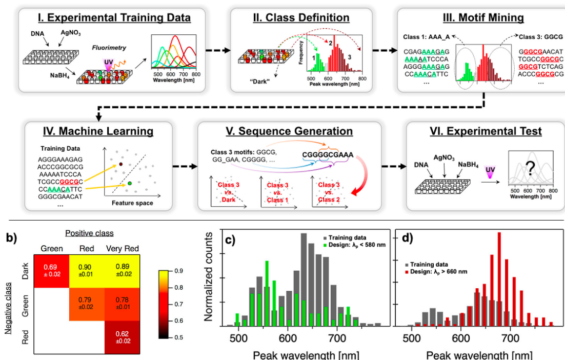
Fig. 7 ML-guided design of Ag N -DNAs with fluorescence emission in specific spectral windows. 71 a) Schematic of ML workflow. b) Cross-validation scores of one-versus-one SVMs for each color class pair. c,d) Adapted from Copp, et al., 71 with permission from the American Chemical Society. Copyright 2018.
