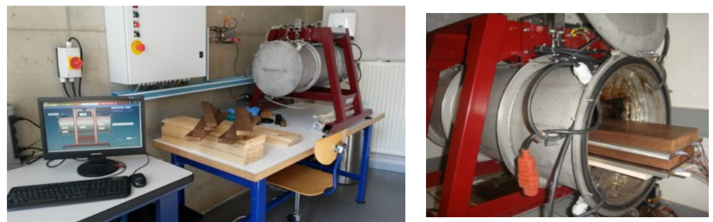
Figure 1. Conductive vacuum reactor.
