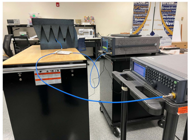
FIGURE 13. Tx-Rx isolation testing with active measurement.
