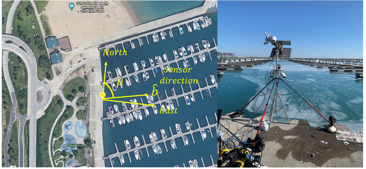
Figure 3: Left: Google Map satellite image of sensor location for data campaign (Lake Michigan Test 11). The yellow arrow defines the boom direction \hat{b} . Right: Photo of the experiment hardware setup, actual picture of the tripod, which is setup on the Lake Michigan 11.
