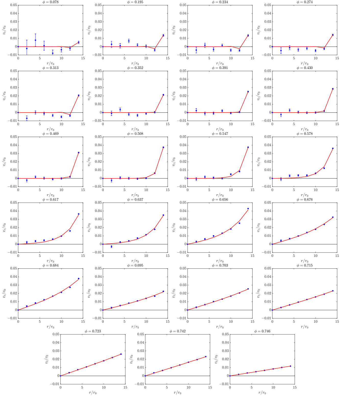
Figure 9. The measured velocity profile for the various area fractions ranging from dilute gas to dense crystal, and corresponding fits to coarse-grain model.
