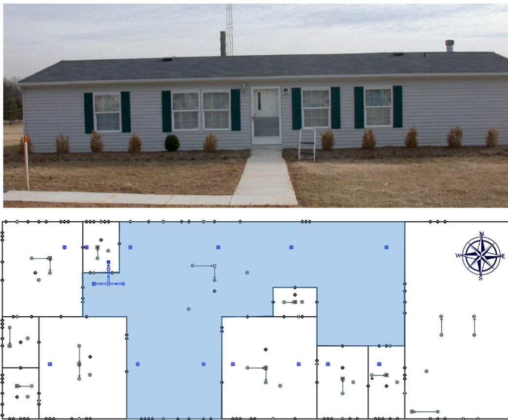
Fig. 2. Building layout and the CONTAM model with window openings (Rim et al., 2013a).
