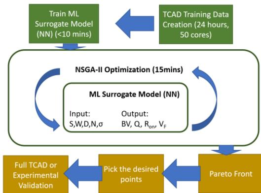
Fig. 6. The rapid inverse design framework. Rapid-TCAD is used to easily and randomly generate 266 sub-optimal structures. They are used to train a NN as the surrogated model, which will be used to find the Pareto front to discover structures with more superior performance without human expertise. The time used in each step is shown. Due to the rapid BV simulation and the use of Pareto front, inverse design and optimization can be finished in 24 hours.
