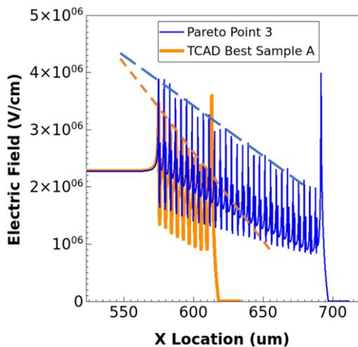
Fig. 10. Electric field distribution cutting at the junction along the white dashed line in Fig. 1 at breakdown for the TCAD Best Sample A (BV  $\sim$  -1350V) and Pareto Point 3 (BV  $\sim$  -1995V). Dashed lines are guidance to show that the Pareto Point 3 is more effective in smoothing the E-field.
