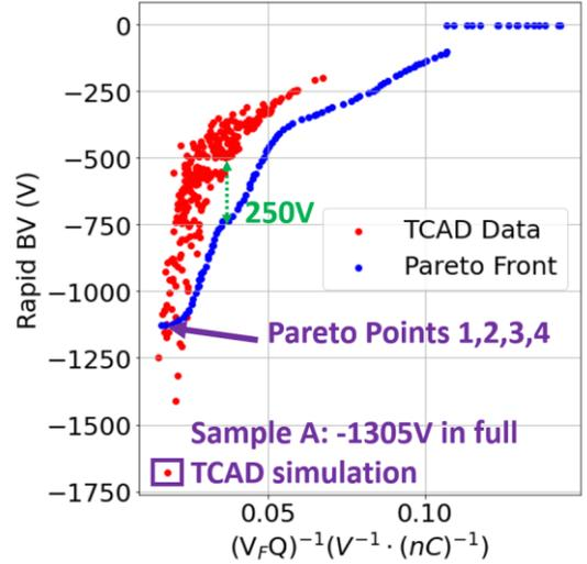
Fig. 7. Distribution of the rapid-TCAD training data and the optimized Pareto front in a BV vs.  $(V_F Q)^{-1}$  plot. Note that the BV are obtained in rapid-TCAD simulation. The maximum BV obtained is only -1305V when the structure is simulated in full-TCAD simulation in Sample A.
