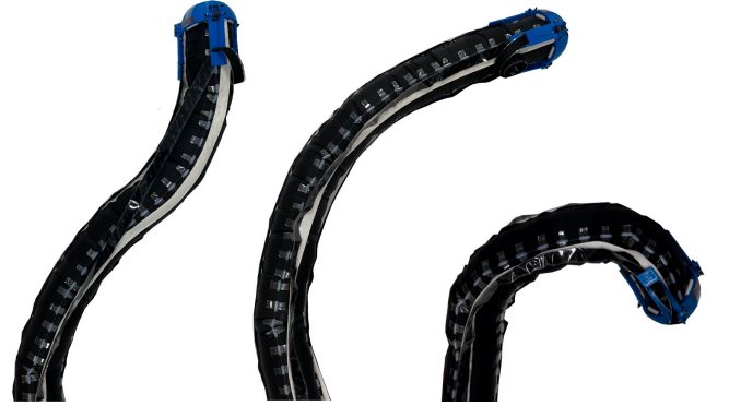
Fig. 1. Photos showing various final robot configurations possible with our proposed shape locking design.
