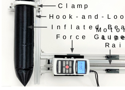
Fig. 7. Experimental setup to measure the beam stiffness of locked and unlocked inflated beams.
