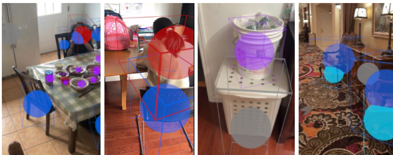
Fig. 7 Examples of AR visualization of 3D object detection results. Blue represents the chair; red represents the person; purple represents the cup, bottle, and bowl; and gray represents the unknown object
