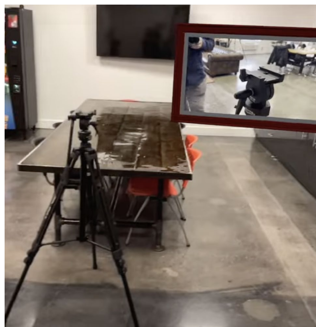
Fig. 8 AR instruction example. The AR frame displays a video showing the user how to attach the camera to a tripod
