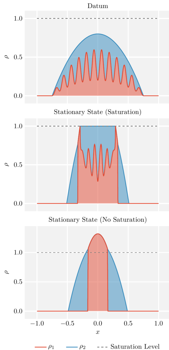
FIG. 6. Stationary solutions of (4.7) in one dimension. \Omega = (-1, 1) , \alpha = 1 , D = 0.1 , C_1 = 4 , C_2 = 2 , \Delta x = 2^{-8} , and \Delta t = 0.1 . Top: datum (4.8). Middle: “frozen-in-place” stationary state with saturation effects. Bottom: segregated stationary state without saturation.
