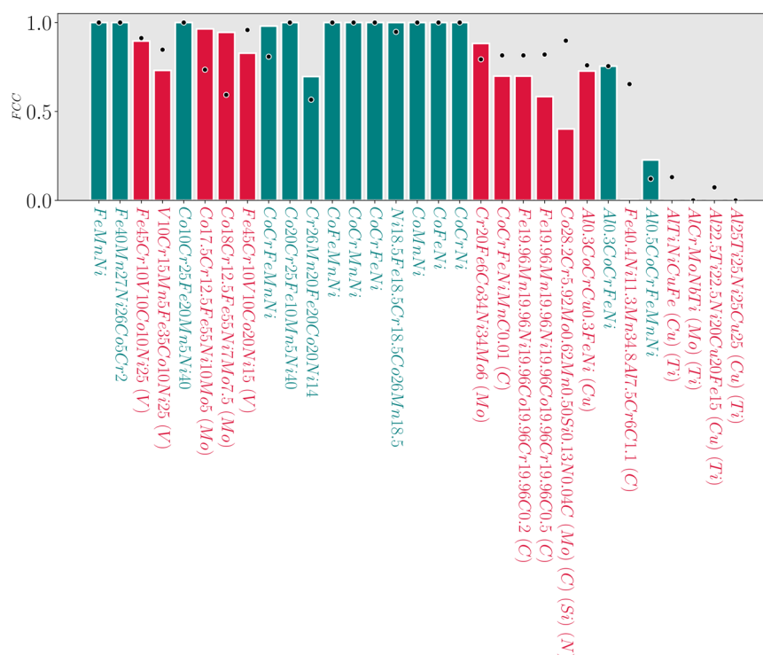
Fig. 8 FCC prediction. DNN regressor predictions for the FCC phase in alloys experimentally characterized as single FCC phase at annealing temperatures of 800 °C or higher. Those alloys with all elements considered in the training system and those which are not, are colored green and red, respectively. Labels for the alloy correspond to the stoichiometry of the alloy and in parentheses the extra elements not considered in the training. Black dots represent the FCC phase fraction prediction using Thermo-Calc single equilibrium running on the TCHEA5 database.
