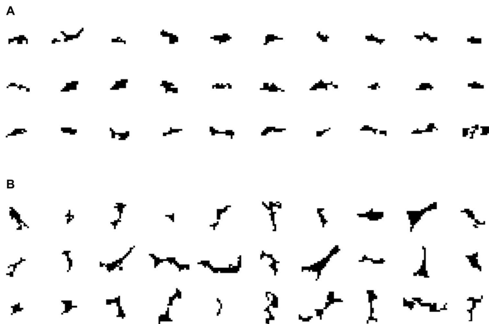
Fig. 7. Examples of critical and noncritical voids identified from the saliency map visualization. (A) Critical voids. (B) Noncritical voids.
