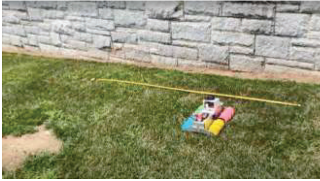
Fig. 8. Lateral Motion on Grass Slope with PLA screws
