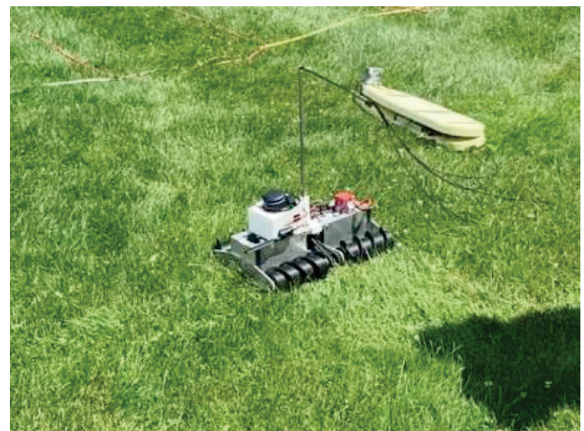
Fig. 1. Screw-Bot and MFAM testing Setup
