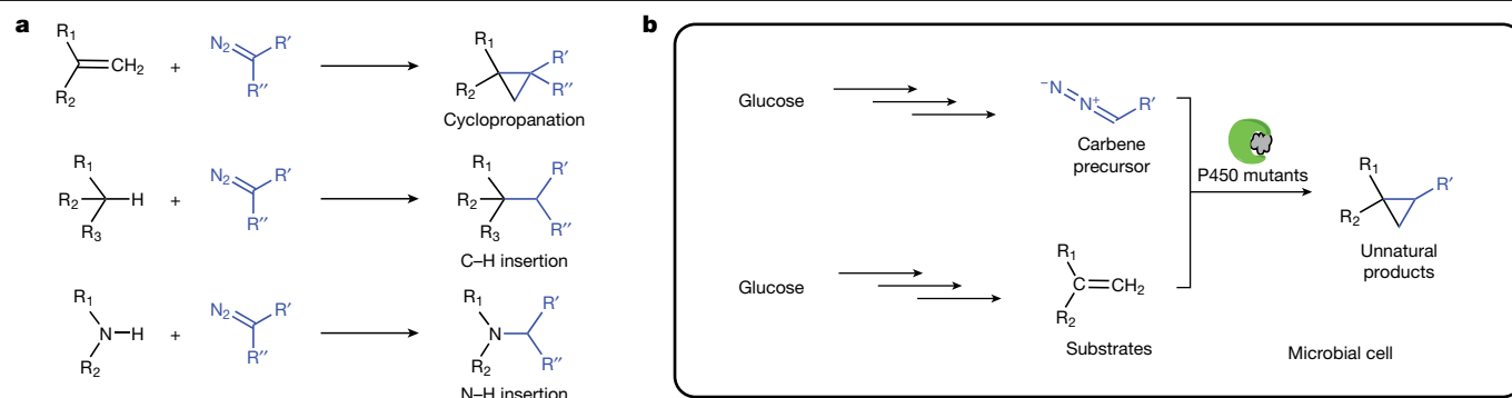
Fig. 1 | Carbene-transfer reactions for biosynthesis. a , Examples of recently developed carbene-transfer reactions catalysed by engineered cytochrome P450s 14 . b , Schematic for integrating carbene-transfer reactions into biosynthesis with all components in the reaction produced by microbial cells.
