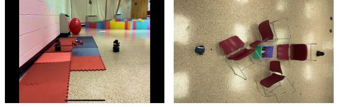
Figure 5. Sample implementation of LOS (image on the left), and NLOS (image on the right) communication scenario with a Duckiedrone and two turtlebots.
