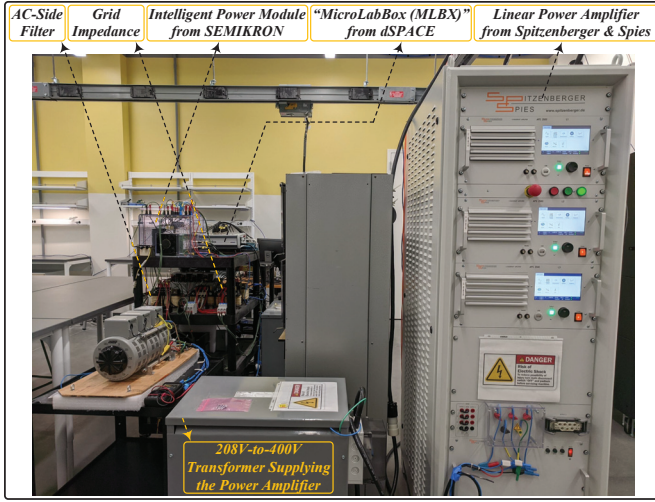
Fig. 4. Test rig employed in the experiments conducted in the Laboratory for Advanced Power and Energy Systems (LAPES) at Georgia Southern University—where the test rig has been housed.
