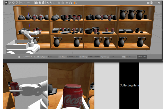
Fig. 1: Experimental Setup. The top figure shows the world view of the environment available to the human supervisor. The bottom left and middle figures show the local view and end-effector view used by the human during teleoperation. The bottom right figure shows the operation status. The setup uses ROS-Gazebo [25] and resources available in [26], [27].
