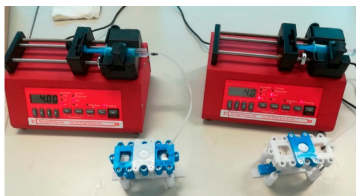
Figure 13. The skin-on-a-chip is developed for monitoring skin toxicity. (A) Schematic and actual image of the skin-on-a-chip. (B) Biomarker expressions by the cells in the skin-on-a-chip in different groups. The figure is reproduced from the work [121].
