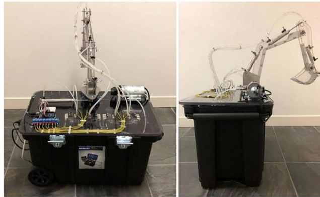
Figure 2. Electrically Actuated Hydraulic Arm: An Interactive Tool for improving student's learning [25]
