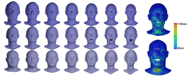
Fig. 9 Tangent PCA for a set of parametrized surfaces. On the left we display the first three principal component geodesics of a training set. On the right, we display a reconstruction of two elements from a separate testing set, where each vertex is colored based on the Euclidean error of the reconstruction
