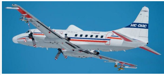
FIGURE 5 Picture of the NRC Convair-580 aircraft with some of the complementary instruments seen underwings.
