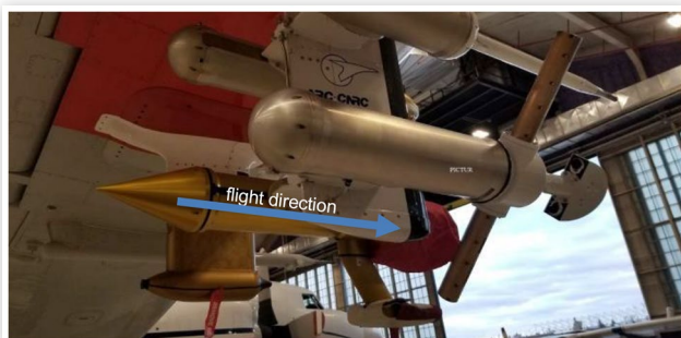
FIGURE 2 An image of PICTUR integrated on the NRC Convair-580 aircraft, underwing Starboard Outer Lower (SOL) position.
