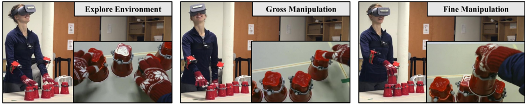
Fig. 2. A representation of the experimental paradigm. The three images show the sequence of actions the subject uses to stack a cup while performing the experiment.
