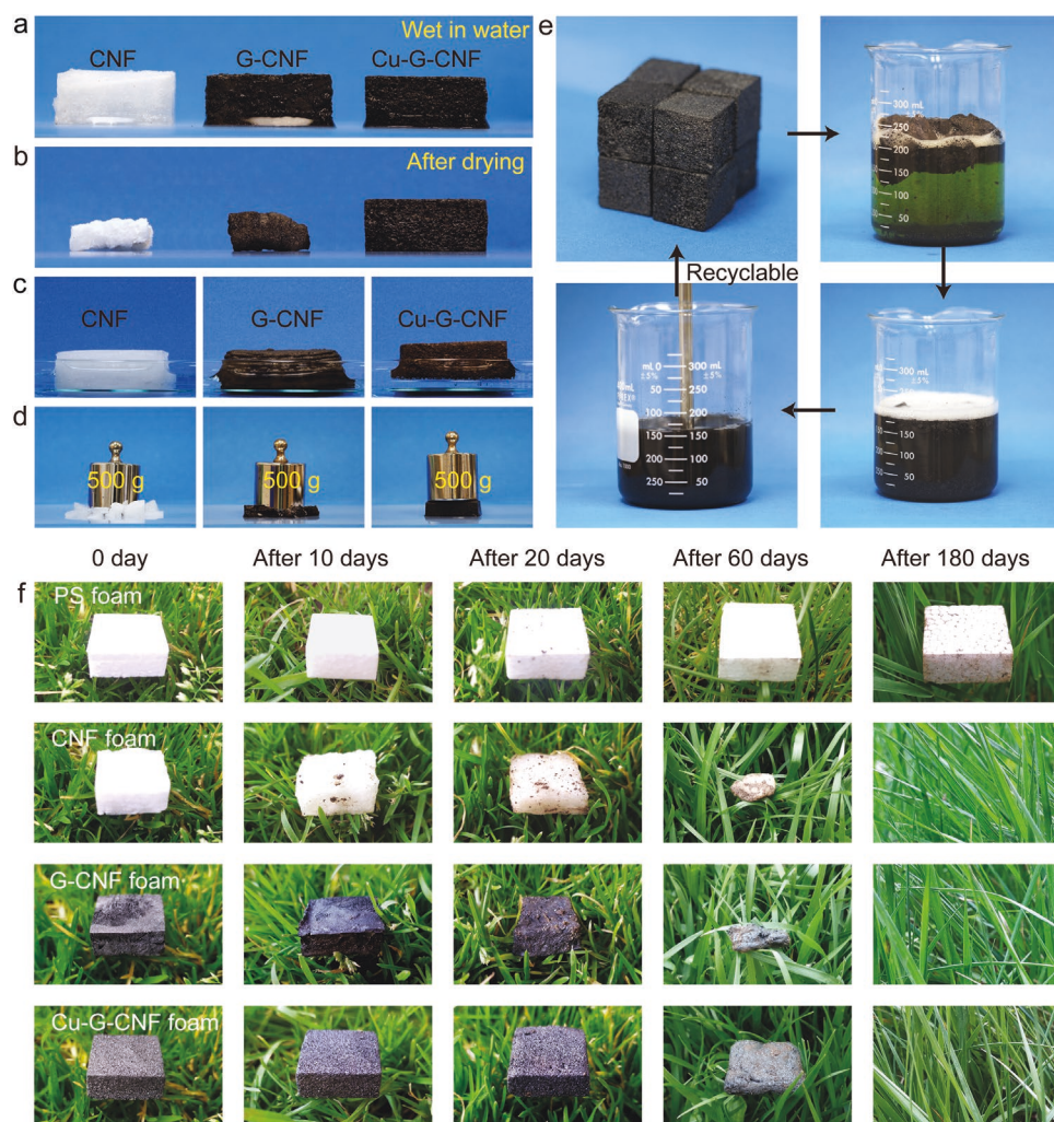
Figure 5. The demonstration of the water stability, recyclability, and degradability of the Cu-G-CNF foam. Water stability of the CNF (left), G-CNF (middle), and Cu-G-CNF (right) foams: Shape retain ability in water, photographs of the foams in a) fully wetted state, and b) after drying. The CNF foam and G-CNF foam shrink significantly, while the Cu-G-CNF foam can retain its shape well. c) Photographs of the CNF foam (left), G-CNF foam (middle), and Cu-G-CNF foam (right) soaked in water. d) Behaviors after compression. CNF and G-CNF foams were easily damaged under the same pressure (the poise is 500 g); on the contrary, crosslinked G-CNF foam kept its 3D structure. e) The recyclability of the Cu-G-CNF foam. f) The degradability of the PS, CNF, graphite-CNF, and Cu-G-CNF foams.
