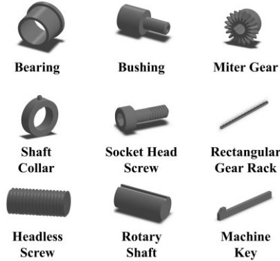
Figure 2. Example 3D CAD models and part function classes
