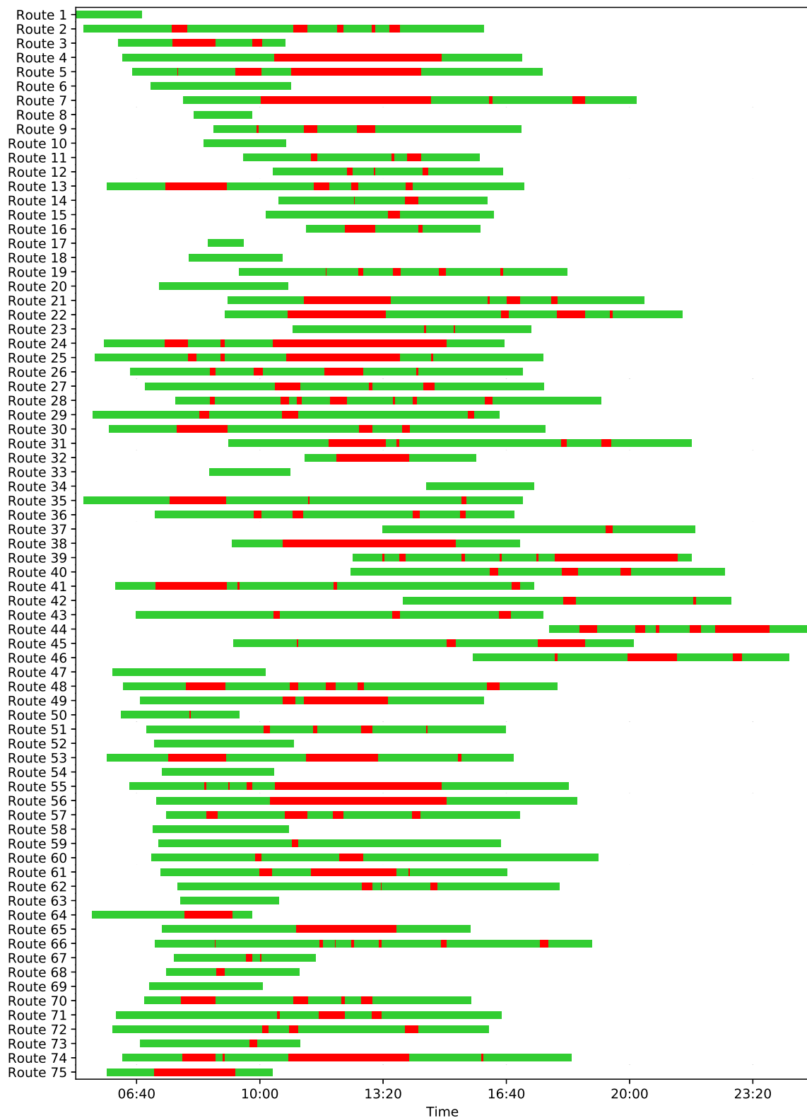
Fig. 5. Schedules of MRMS routes. Green and red colors indicate spans of driving and idle periods. (For interpretation of the references to color in this figure legend, the reader is referred to the web version of this article.)
