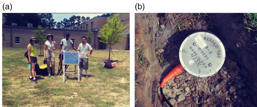
Figure 2. (a) Field installation of a seismic station in the Summerville High School (YH.SFHS) and (b) L22 short-period seismometer in position. The color version of this figure is available only in the electronic edition.
